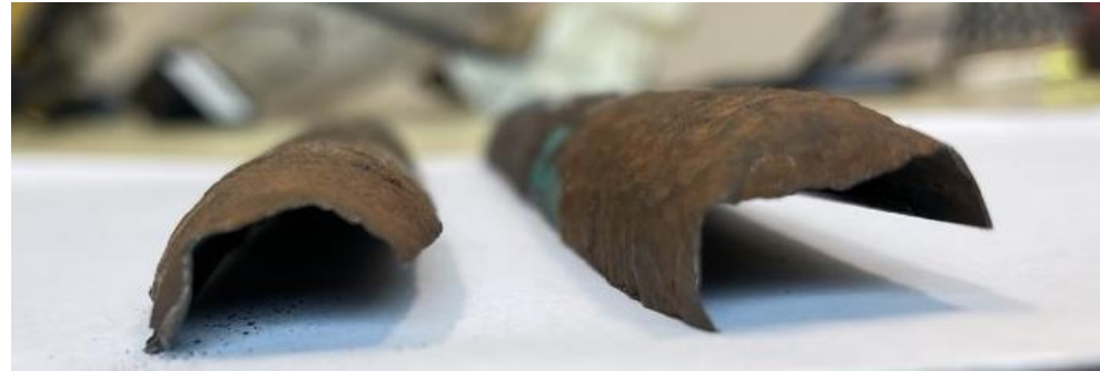
2. Tube profile at sheared end (near tubesheet)
