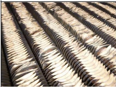
Fig. 12: Tube fins Almost fins were slightly deformed at top side.
