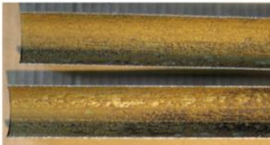
Figure 5 - Severe erosion corrosion of 25.4 mm OD 6620/22 Cu-Ni-Pb-Mn in a dump condenser due to syphonic air release
